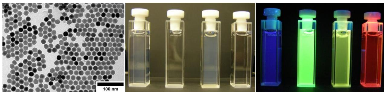
Figure 1: Rare earth ions dopant variation results tuning multifunctional properties. TEM of core@shell upconversion NPs having magnetic and optical properties (left); downshifting nanoparticles in water, under daylight (centre) and under UV light (right).
